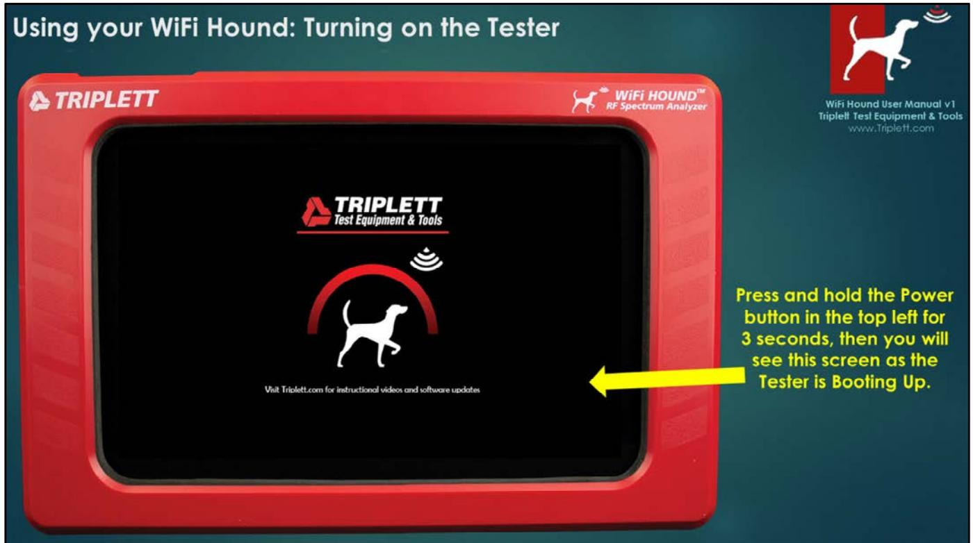
As mentioned earlier, if you press the power button and the Volume control at the same time by accident, you will enter into the Android OS control screen. The only way to get out of that screen is to use a paperclip to do a Hard Reboot. If you press the power button and see the above screen, you are in the correct place. Give the Tester a minute to fully boot up.
