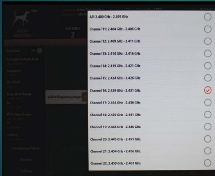
In this example, if you had selected Zigbee in the Channel Width options, you would then see this set of Zigbee-specific Channels. You can select a channel to apply the filter.
