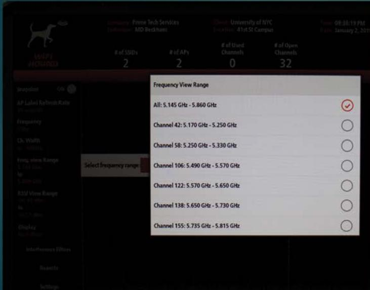
If you selected the 80MHz Channel Width, then these bonded channels will show as options for filtering.
