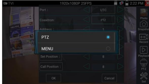
Input calling dome camera menu address code, after finishing the parameter settings, you can press the key “Enter” or click the icon
