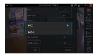
Input calling dome camera menu address code, after finishing the parameter settings, you can press the key "Enter" or click the icon 🔵 to call the dome camera menu.
