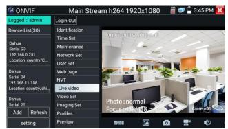
While in the "Live video" menu, click "Video Menu" at the top right of the image to access the following tools: Snapshot, Record, Photo, Playback, Lens simulation, PTZ and Settings.
