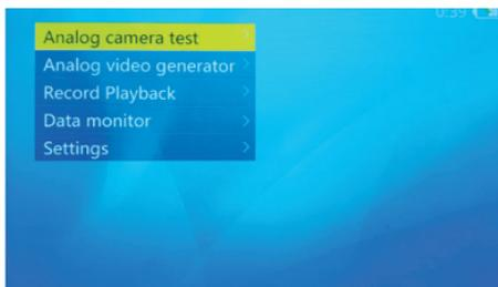
You can navigate this screen using the **Up or Down Arrow Keys**. Once you have highlighted the function you want to use, press the **Right Arrow Key** to go to the Interface Screen for that feature.
