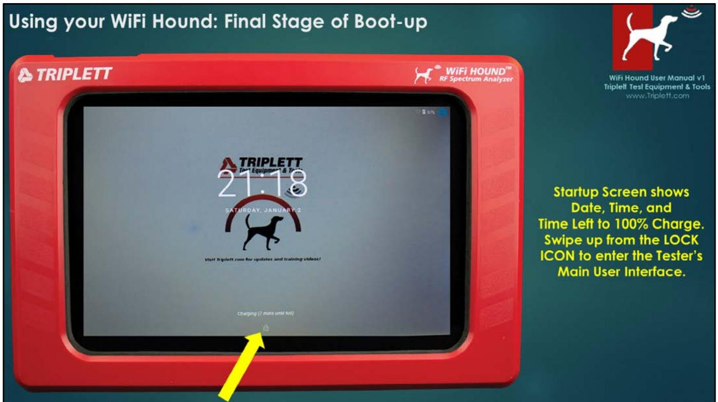
This is the WiFi Hound Startup Screen. This is the screen you will see once the unit has completed its boot-up process. Swipe up from the Lock icon to begin using your Tester.
